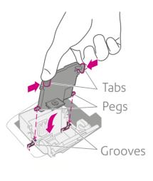
d. Squeeze the tabs and slide the printhead pegs into the lower set of grooves.
