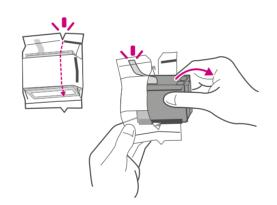
e. Keep squeezing the tabs and push the printhead flat against the make sure you remove the silwall. The tabs will click open when ver foil strip. placed correctly.
