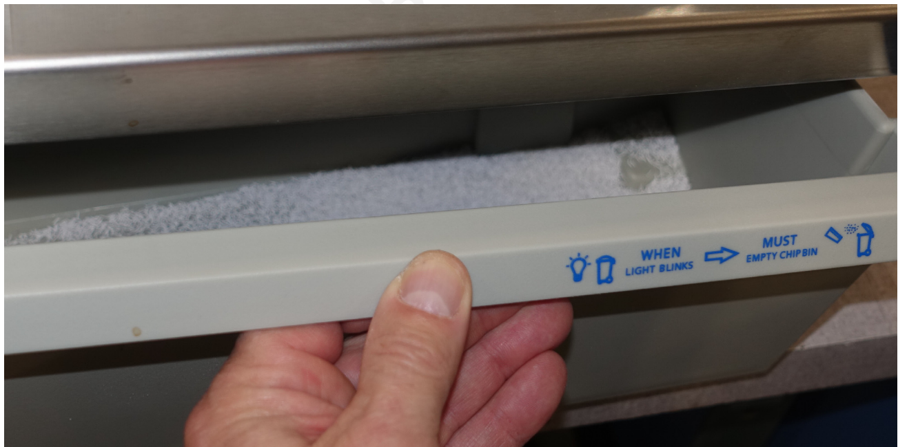
Figure 4-3: Opening the Chip Bin tray
