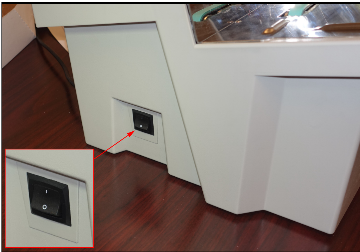
Figure 4-5: AC power switch
