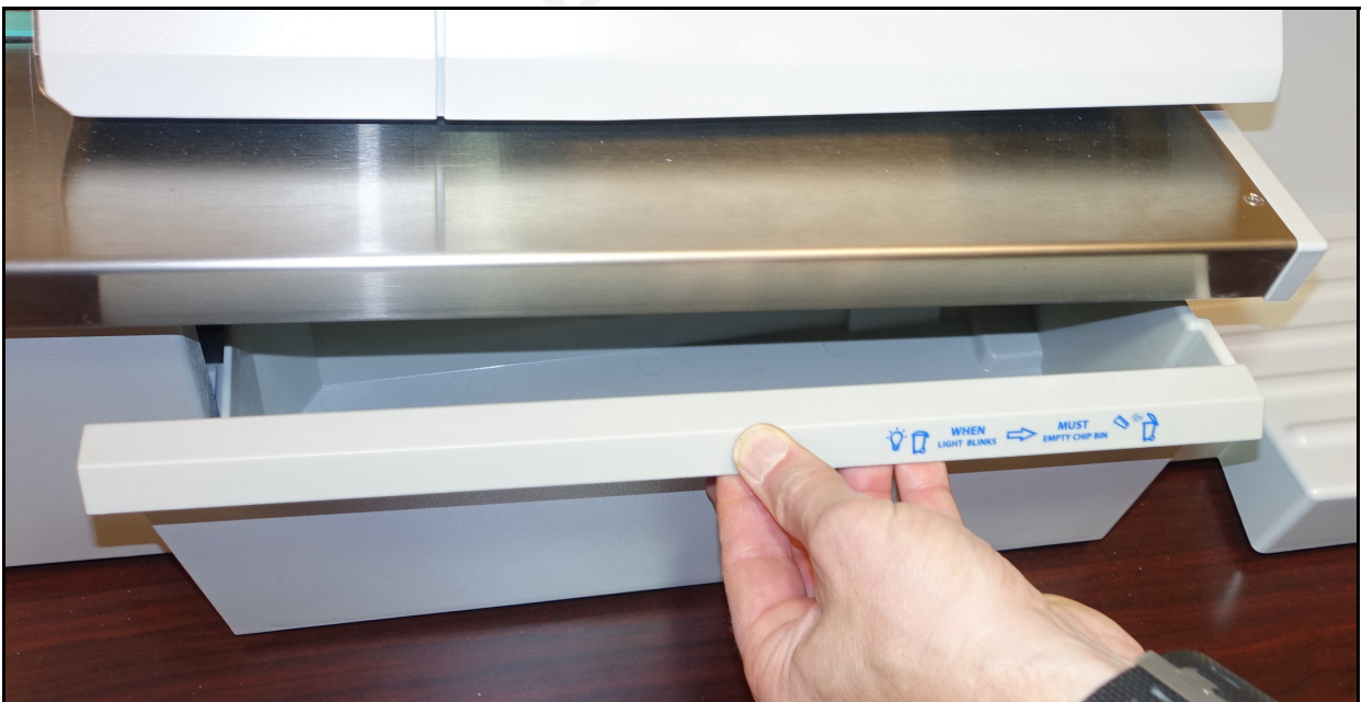
Figure 2-10: Bin tray removal interlock triggering
