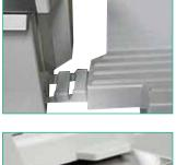
Chip waste is stored for easy disposal. Chip bin full indicator light flashes after 3,500 envelopes are processed.
