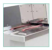
Self-adjusting feeder mechanism enables a wide variety of envelopes to be processed with no tamping
